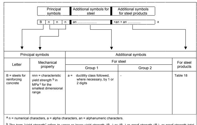
Table 5 — Steels for reinforcing concrete
